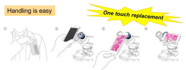
Just replacing regular ocular lens by i-NTER LENS and attach iPhone with attaching case.
